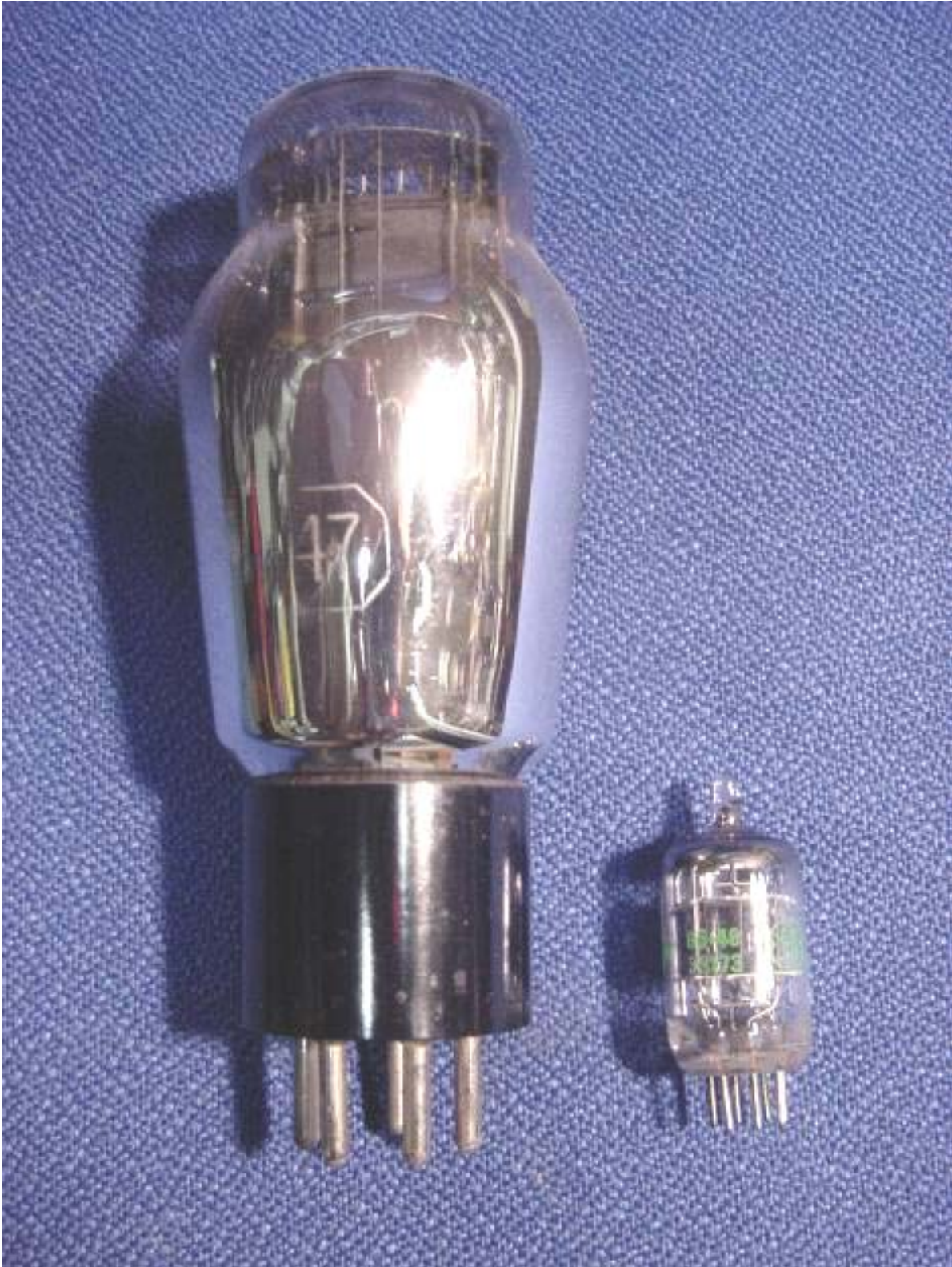
The long and the short of it... a 1930's #42 alongside a 6AL5
